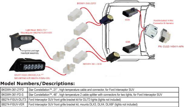
BB274-FISUV-GRL Ford Interceptor SUV headlight bracket kit, mounts DLX3, DLX4, DLX6F in the headlight of 2016 Police Ford Interceptor SUV (lights not included)
